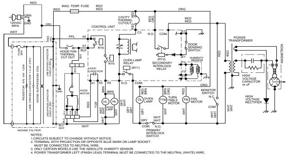
Figure O-1. Oven Schematic-Off Condition
